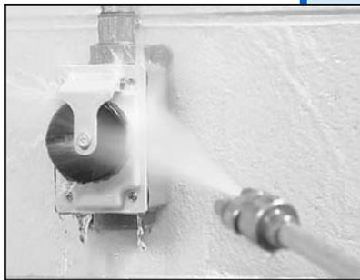
1000 PSI water spray was directly applied at the face of DuraGard receptacles. No damage occurred, and no water penetrated the housing or cord seal. DuraGard plugs, connectors and receptacles are designed to withstand water spray test at 1000 PSI. No extra cost boots or adapters required.
